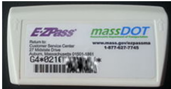
Figure 1: Active RFID Tag – E-Z Pass toll payment Source: Mikeettm used under CC BY
